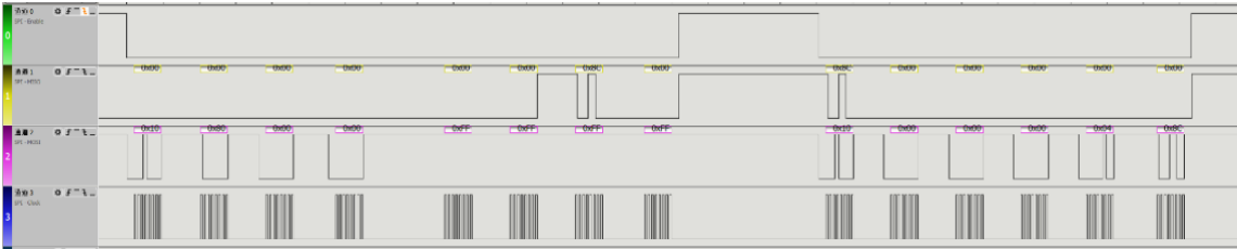
Fig. 12 Timing diagram of RT mode start configuration for MK64F12 version
