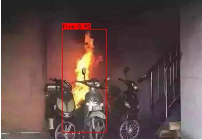
Figure 1. Example of flame image detection
